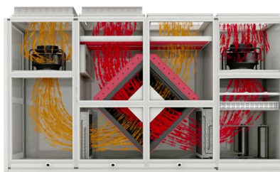
Operation @ high outside air temperatures
