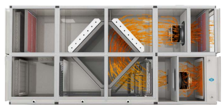
Recirculation only, e.g. night operation
